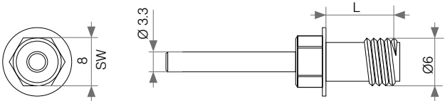
Fig. Clinch bolt TU-S6.0x9 - Construction and dimensions (mm).
